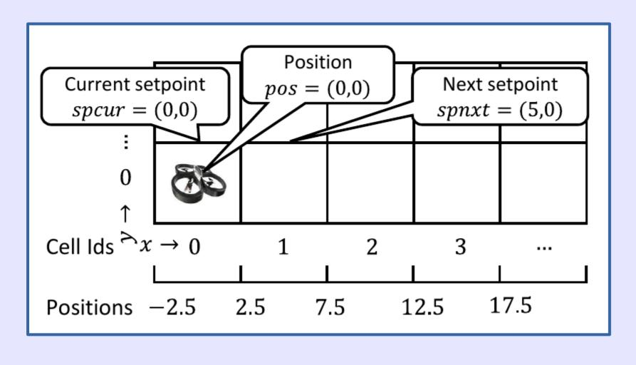
Consider a distributed quadcopter system where each agent moves in a 2d world. Each helicopter has continuous dynamics. We want to prove distributed, end-to-end collision avoidance.
