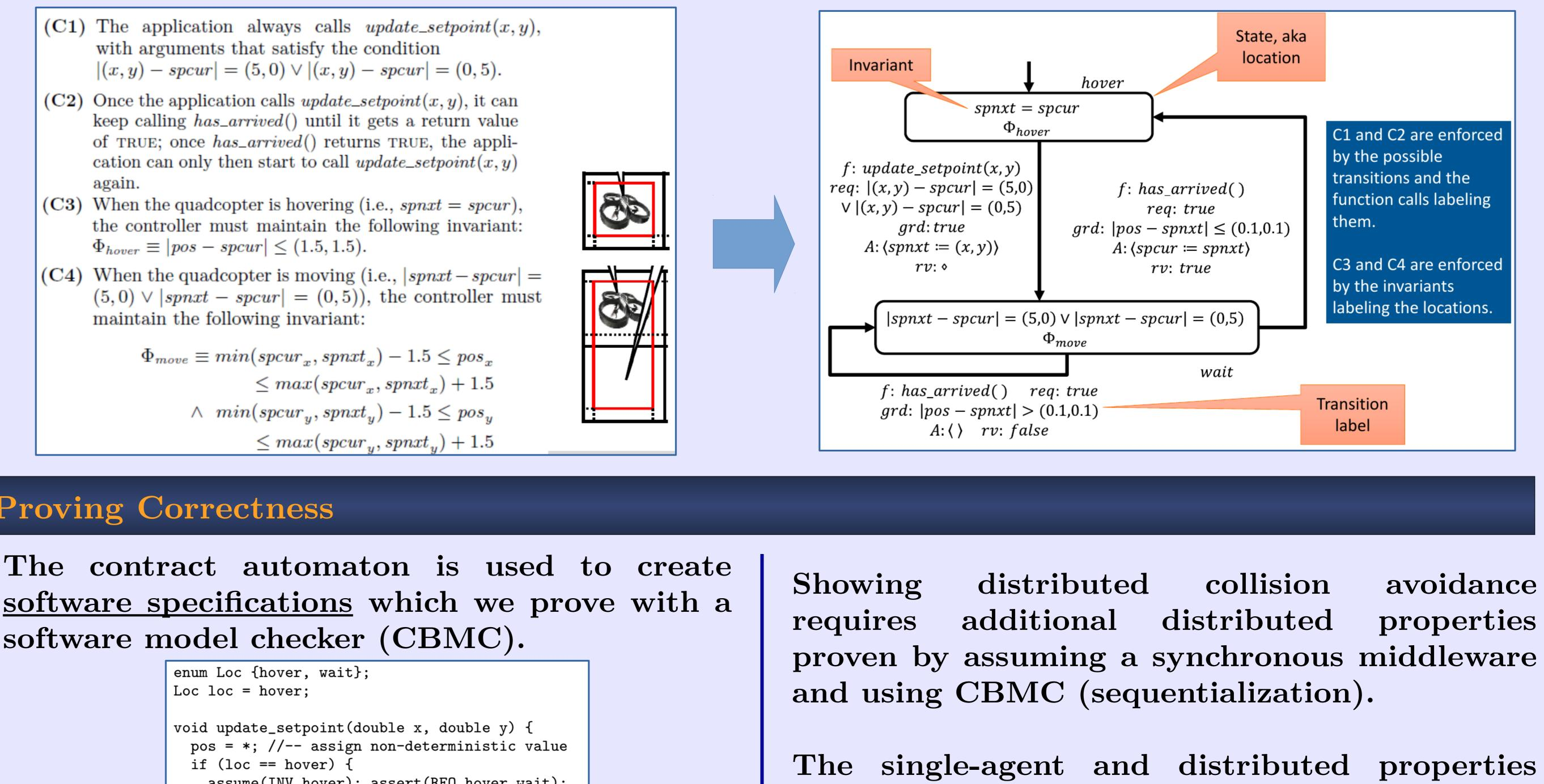
The single-agent and distributed properties can then be composed into an SMT problem to check if collisions are possible, which is discharged using Z3.
