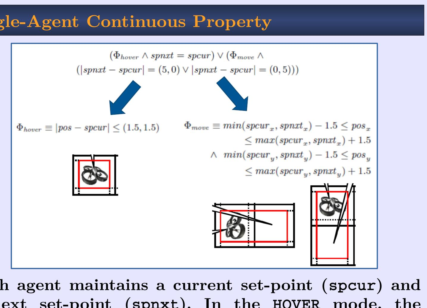
Each agent maintains a current set-point (spcur) and a next set-point (spnxt). In the HOVER mode, the agent must stay near spcur. In MOVE mode, the agent must stay near the set-points' connecting line.
